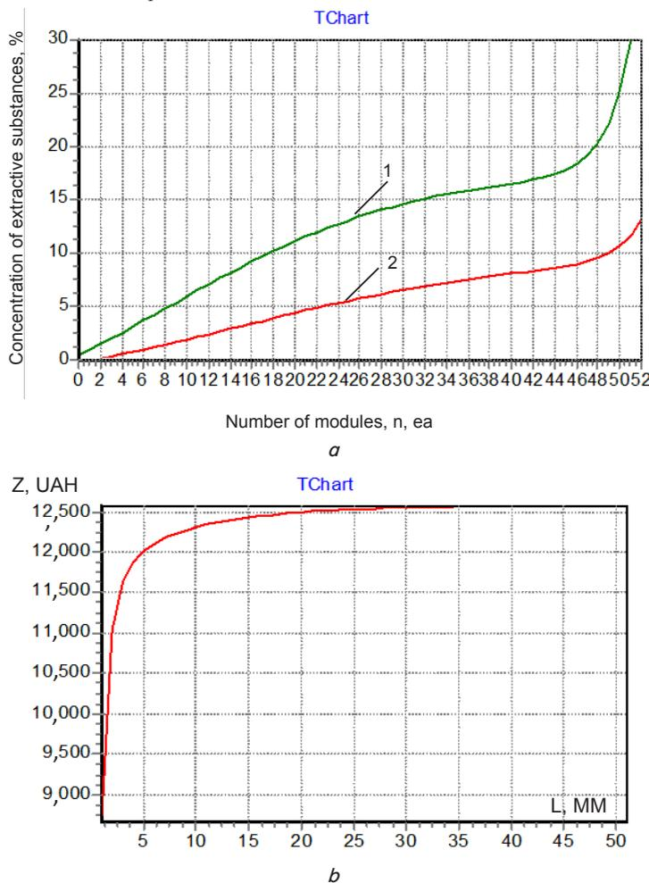
Fig. 12. The computer modeling:  $a$  – the distribution of the concentration of extractive substances according to the modules corresponding to the local maximum of  $Z$
