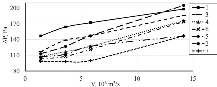
Fig. 6. The hydraulic characteristics of the cassettes of the microwave extractor: 1 – less than 0.8 mm; 2 – 1...2 mm; 3 – 1/2 of coffee beans; 4 – 2...2.5 mm; 5 – 1/4 of coffee beans; 6 – 2.5...3 mm; and 7 – whole coffee beans
