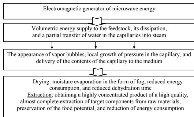
Fig. 1. The thermophysical model of the mechanism and effect of barodiffusion
