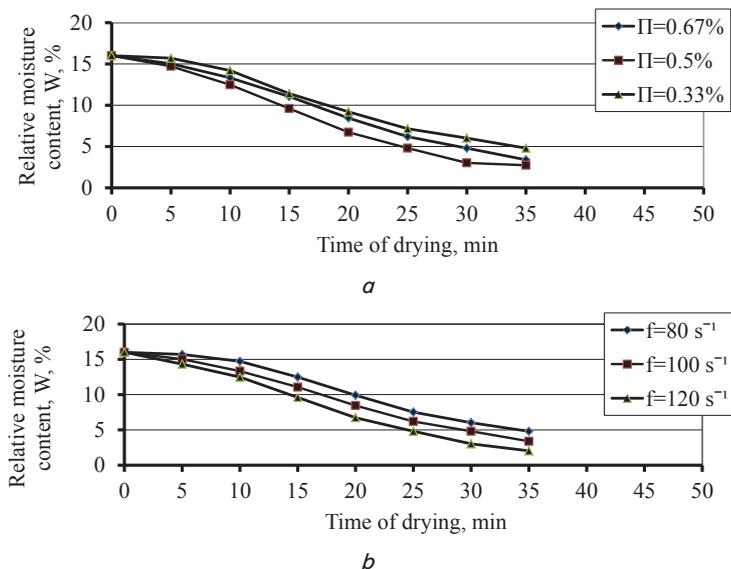
Fig. 8. The kinetics of the drying process of sunflower in the vibrodryer under the following changes: *a* – the container loading; *b* – the vibration frequencies
