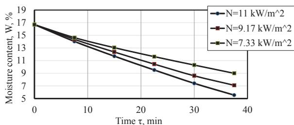
Fig. 10. The drying lines for sunflower seeds on an IR belt dryer
